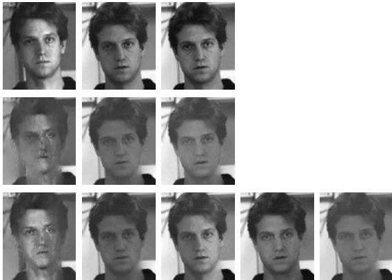
Figure 4. Some examples of the recovered reflectance images. The images in the first row is the reflectance images recovered by median operator with three input images, the images in the second row are the results of the min operator with the same input of the first row. The images in the third row are the other results of min operator with two or four input images (the last one).
