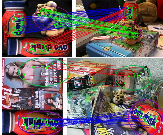
Figure 7. Multiple common patterns detection under different scales and large deformation. For clarity, only parts of correspondences are plotted.
