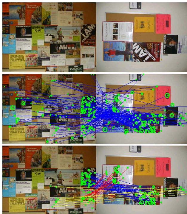
Figure 1. Three common visual patterns detected between two images. All candidate feature point matches after pruning are shown in the middle row, our method can reliably locate all three common visual patterns at different scales and establish spatially coherent correspondences between feature points as demonstrated in the bottom row. For better viewing, please see the original color pdf file.
