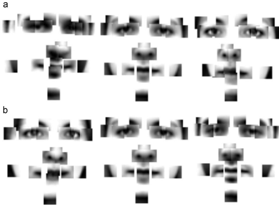
Fig. 1. PCA modes of combined shape and texture variation for CLM face model ( \pm 3\text{std} ).
