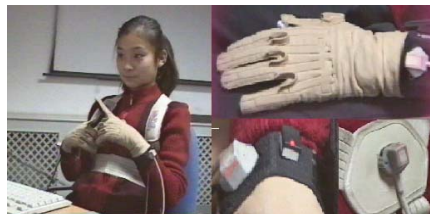
Figure 1. The Dataglove and the 3-D tracker used in our system. Three receivers are fixed on two hands and the back respectively.
