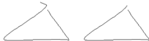
Figure 6. An example of removing the hook at the beginning of the gesture.
