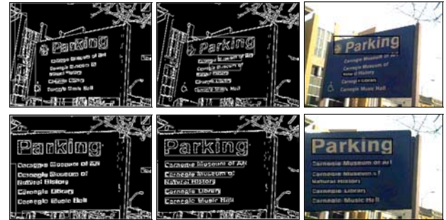
(a) Character candidates (b) Coarse layouts (c) Final results Figure 6. An example of text detection with/ without affine rectification
